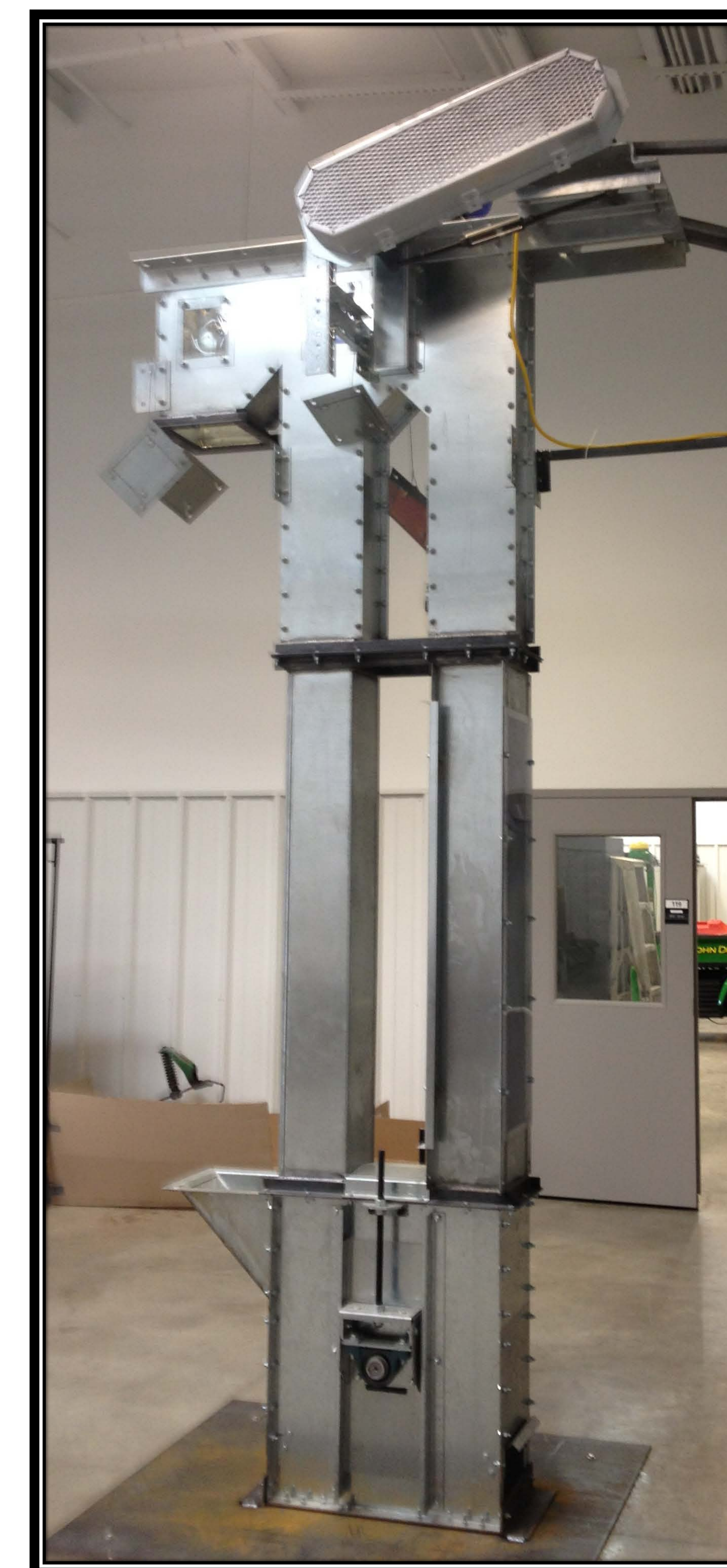
The training module includes the 12' grain leg (above) and the slide show (left) containing instructions on specific components of the leg
